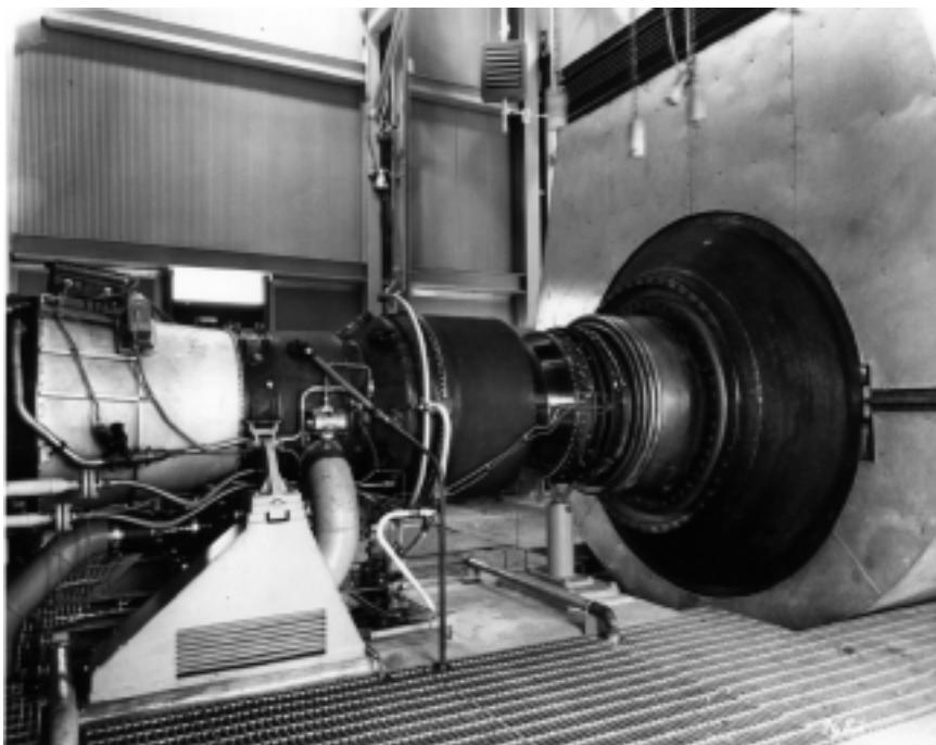
**Figure 1-3.** Courtesy of Cooper Cameron Corporation (formerly Cooper Bessemer Company). Partial view of the Cooper-Bessemer 10,500 horsepower, Model RT-248 gas turbine-compressor at Clementsville, Kentucky. Cooper-Bessemer teamed up with Pratt & Whitney Aircraft to employ a modified J57 jet engine (later identified as a GG3) as the hot gas generator for the RT-248 power turbine. J57 turbojet engines were used extensively on the Boeing 707 jet aircraft.
