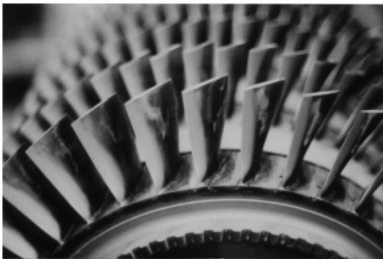
**Figure 12-5.** Carbon deposits distributed across the compressor blades. These deposits extend from the first to the sixth stage blades. 5,000 horsepower gas turbine-generator unit with over 16,500 hours operation.
